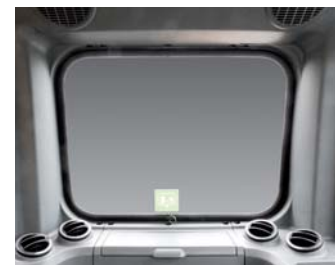
Rear Window Emergency Exit
